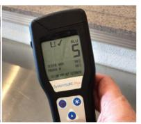
**After Simix:** ATP reading after cleaning with Simix is 5. The CDC accepts ATP readings as an objective measurement of the cleanliness of surfaces. Anything less than 10 is considered sterile in operating rooms, ICU. and sterile services.
